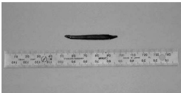
Fig. 1. Photograph of a single crystal ingot of CeNiGe 2 .
